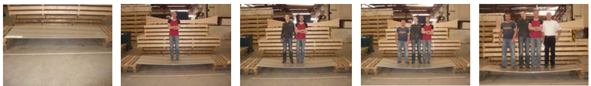
Strength of aluminum honeycomb construction: the "four Dutchman test"
